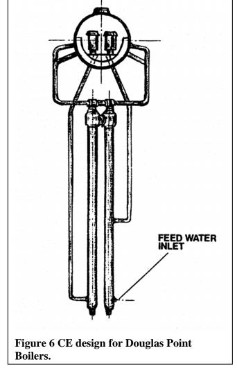
corporation. Thus they used a horizontal fossil-type steam vessel, similar to NPD which was an AECL choice. To meet the CANDU conditions for the steam conditions and cycle parameters they used vertical hairpin heat exchangers with one vertical leg for boiling heat transfer and another vertical leg for the preheater, both joining at the top to form a steam water mixture which
